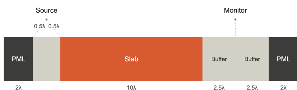
Figure 1: Layout of the 1 Dimensional MEEP simulation domain, established in accordance with best practices for accurate simulation
